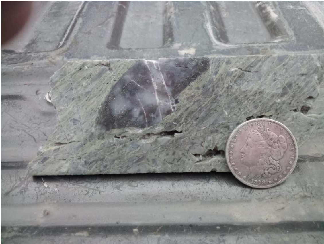
Figure 7.5 - Lapilli Tuff with well-mineralized rhyolite clast
