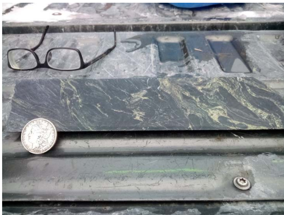
Figure 7.7 - Core from drill hole LS21-015 at 70.4m. Massive, fine crystalline magnetite with interbedded wispy sulphides.
