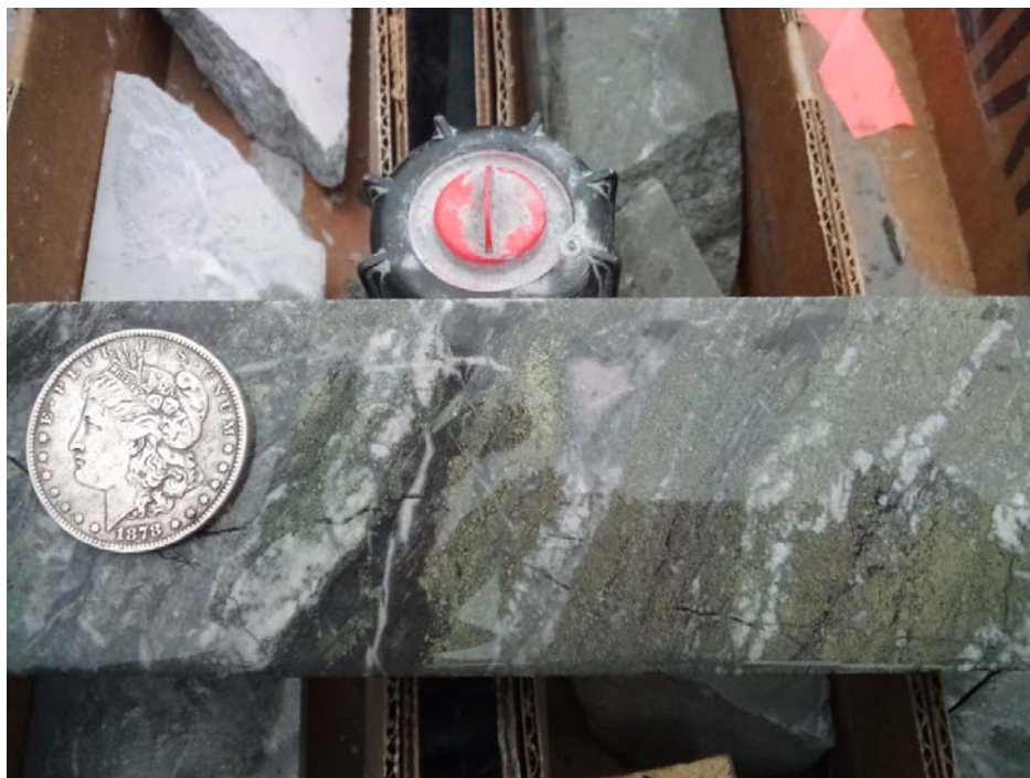
Figure 7.6 - Core from drill hole LS-21-011 @ 124.7m. Bedded massive sulphide with interbedded chert
